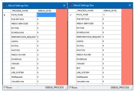
You change the DEBUG\_LEVEL value associated with a process by changing the number in the display grid and pressing Enter.
