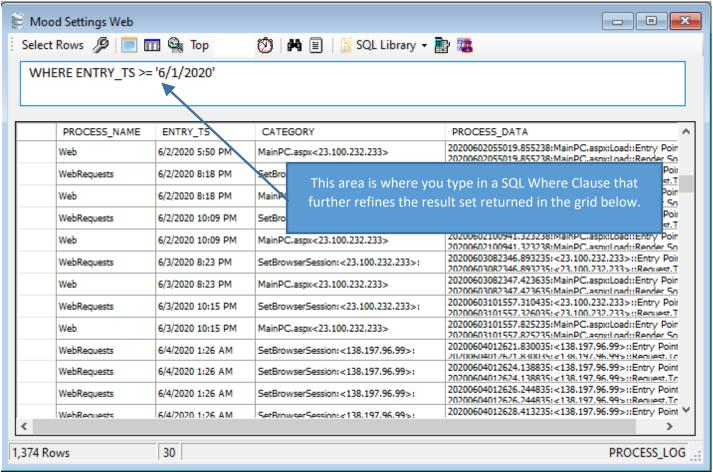
At the top of the window is the tool bar providing access to functionality. Under the tool bar is a textbox where you can enter and issue WHERE Clause SQL Stub Statements. Below the textbox is a Data Grid where the results of the log table select query is displayed.
